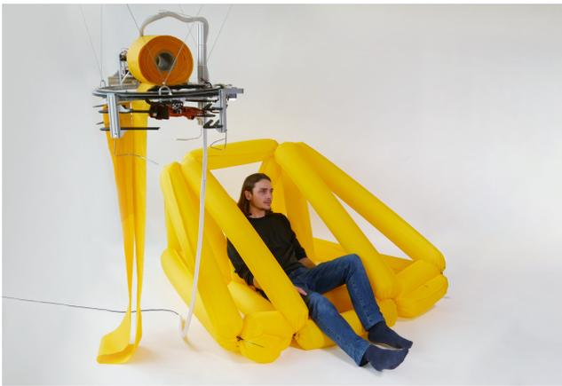
**Figure 7:** During use, we suspend the device to provide space for the dropping tube.
