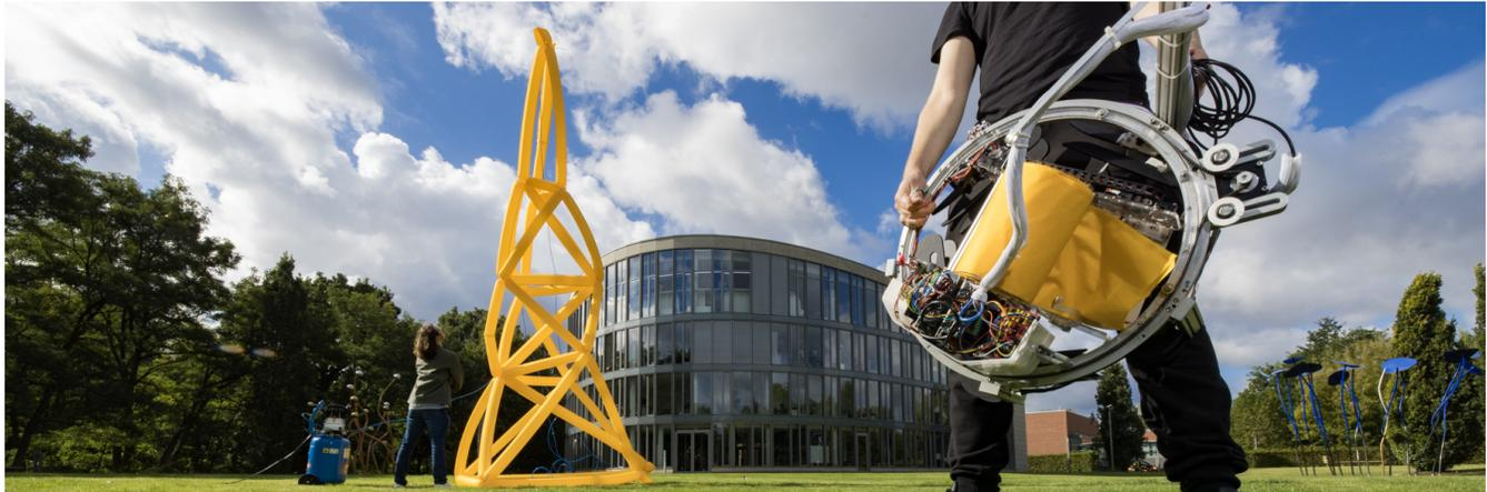
Figure 1: The AirTied device (right) fabricates large truss structures in fully automated fashion, such as this 6 m tower designed to hold a WiFi beacon.
